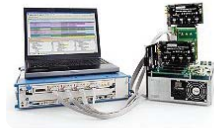
Figure 13. Thoroughly calibrate the device under test (DUT) with Agilent's exerciser.
