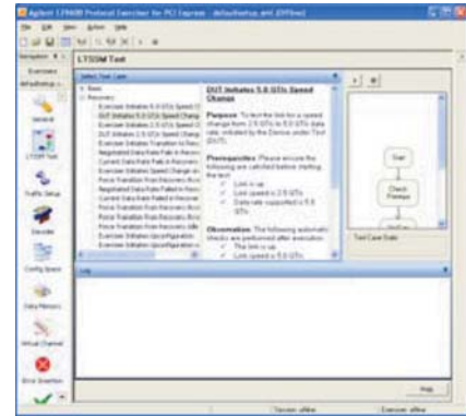
Figure 12. Configuring LTSSM tests is quick and easy with the LTSSM exerciser for PCIe 3.0 and PCIe 2.0
